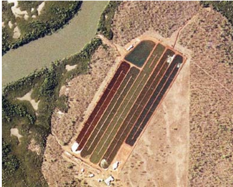
Photo 5.1. Aerial photograph of one of the NT's pond-based barramundi farms. This farm uses a unique 'race track' design for each of the ponds. Total pond surface area is approximately 12 hectares
