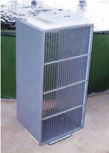
Photo 4.4. (above) Home-made PVC and acrylic grader box. The box floats in the tank (acrylic rods to the bottom) and the fish are added through the open top
