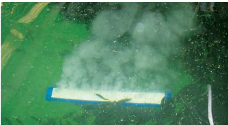
Photo 4.3. Ceramic oxygen stone operating in a barramundi nursery tank. The stream of oxygen from the stone can be clearly seen
