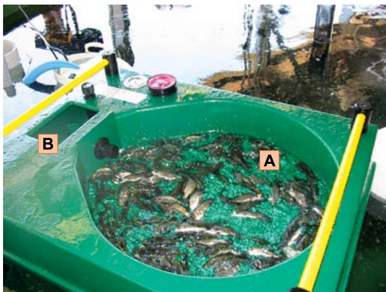
Photo 4.6. Impex™ mechanical fish counter. Fish are added to the basin (A) and flushed from here, down past the sensors (B), and counted
